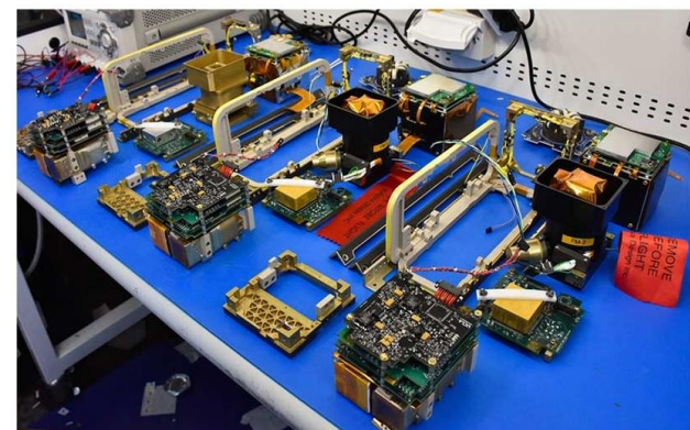
Some photographs of the ELFIN Cubesats with onboard sensors and electronics
