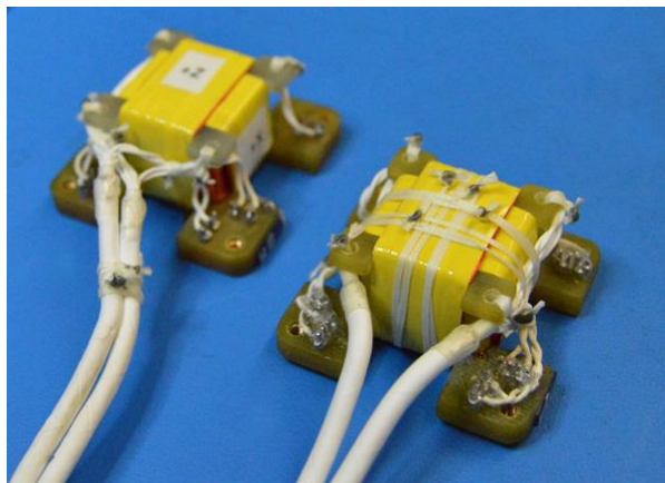
Left: Fluxgate magnetometer sensors to precisely detect magnetic fields Right: Energetic Particle Detector
